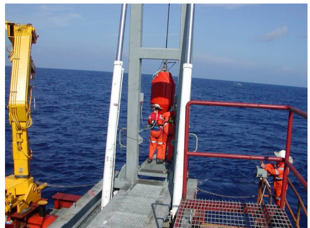
Above: Deploying deepwater floats for umbilical catenary
